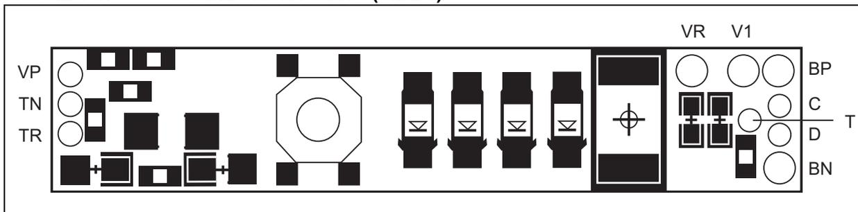
**FIGURE 1-2: BOARD ASSEMBLY (SIDE 1)**
