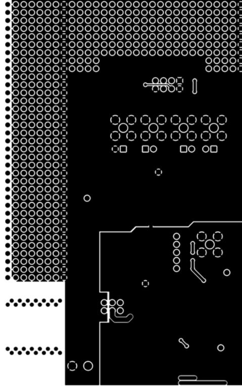
Figure 8. AD7797 Evaluation Board Solder Side Artwork
