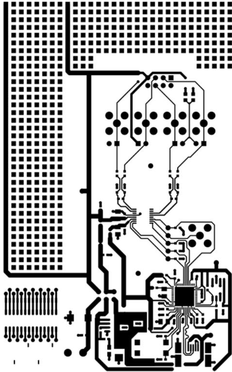
Figure 7. AD7797 Evaluation Board Component Side Artwork
