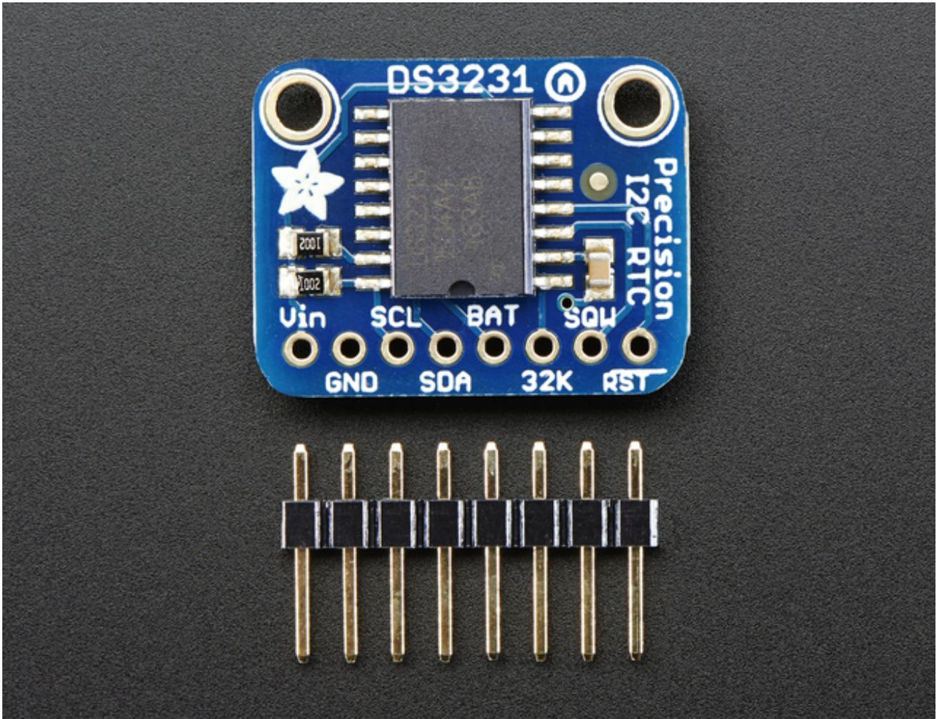
This is the finest RTC you can get, and now we have it in a compact, breadboard-friendly breakout. With a coin cell plugged into the back, you can get years of precision timekeeping, even when main power is lost. Great for datalogging and clocks, or anything where you need to really know the time.
