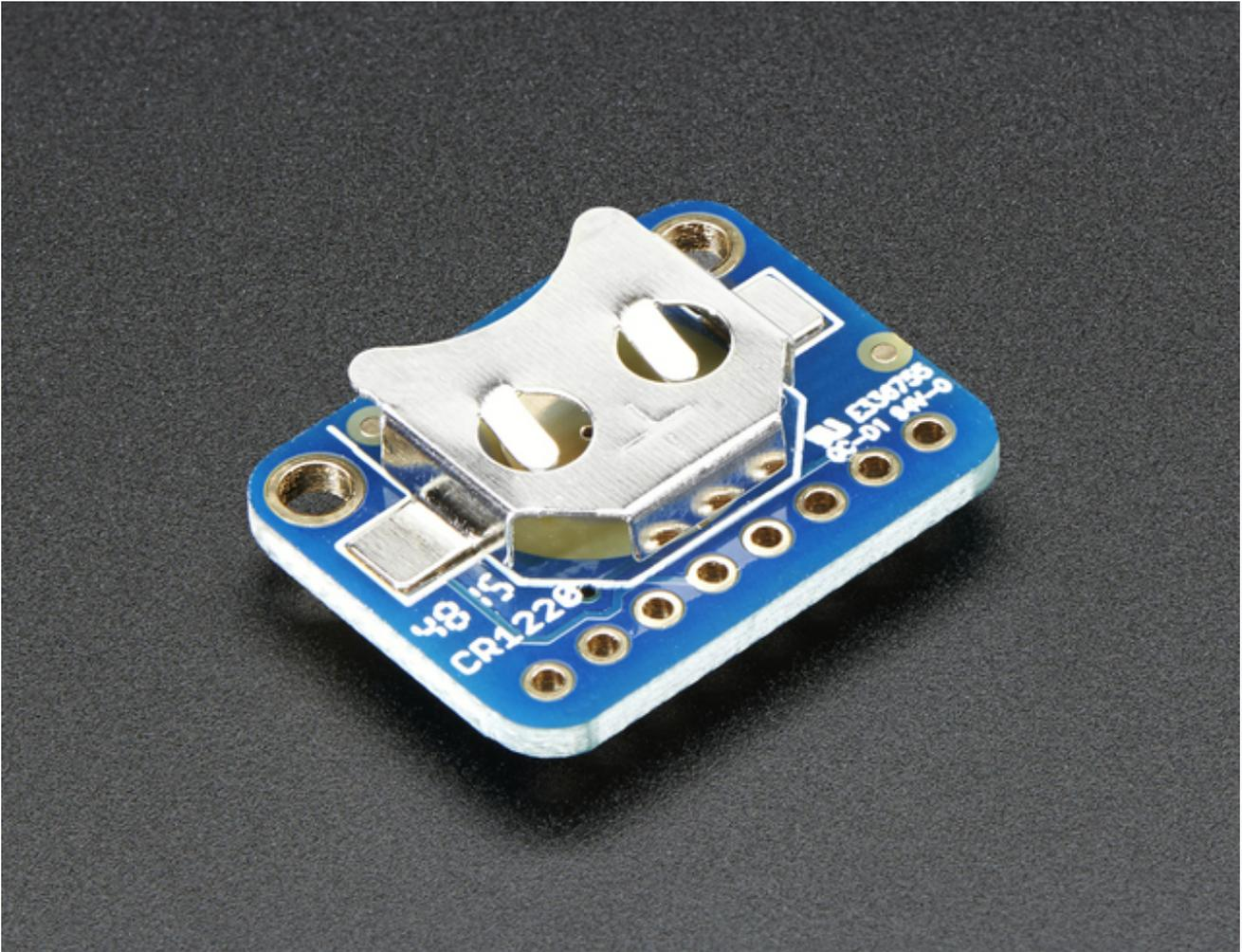
Comes as a fully assembled and tested breakout plus a small piece of header. You can solder header in to plug it into a breadboard, or solder wires directly.
