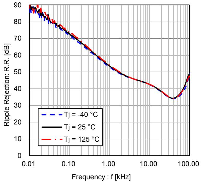
Figure 14. Ripple Rejection (ein=1Vrms, Iout=100mA)
