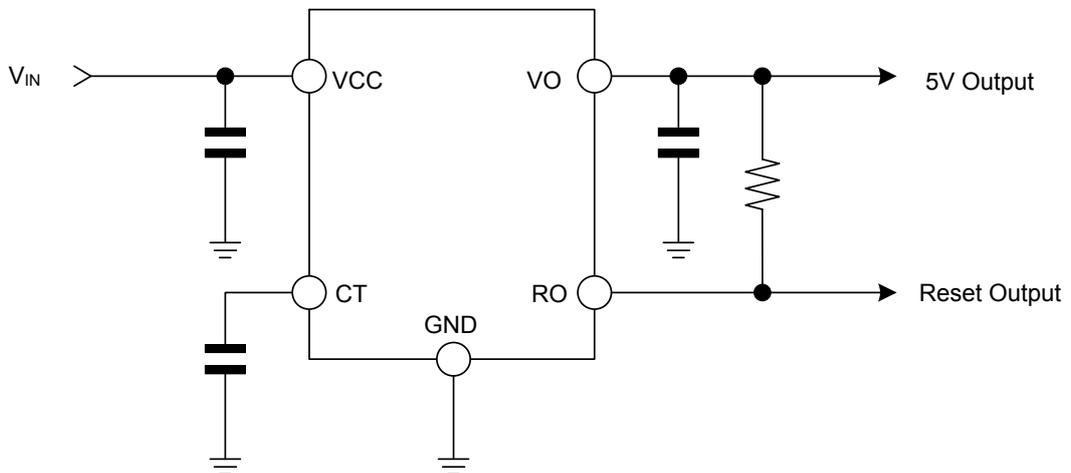
Figure 2. Application Circuit
