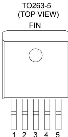
Figure 3. Pin Configuration
