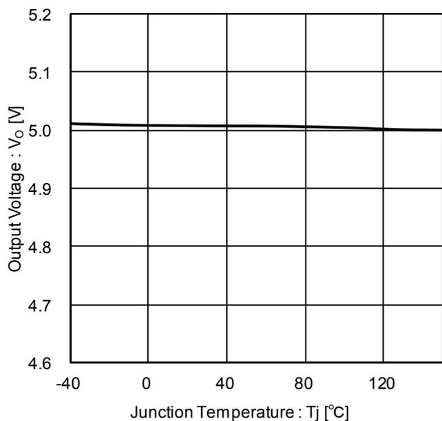
Figure 7. Output Voltage vs Temperature ( $R_L = 1\text{ k}\Omega$ )
