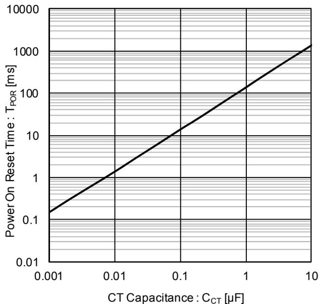
Figure 19. Power on Reset Time vs CT Capacitance
