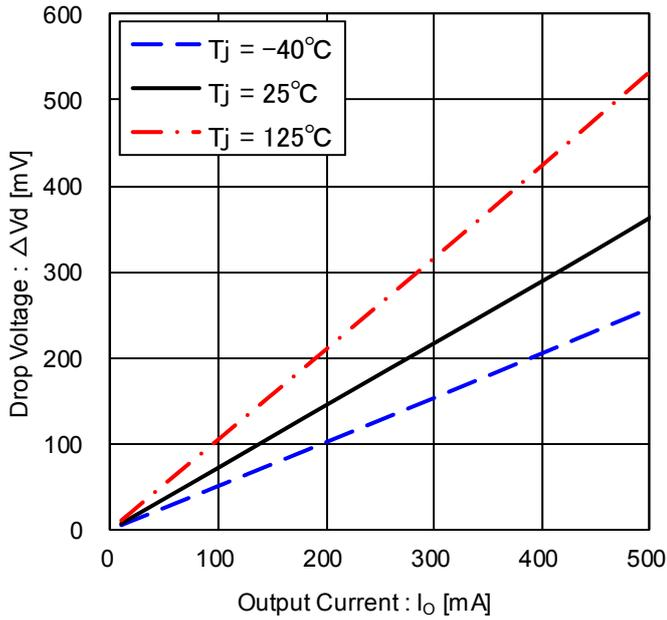
Figure 13. Drop voltage vs Output Current (Vcc = 4.75 V)
