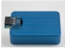
The base station is the hardware between the camera and the PC and it does the deserialisation of the data stream that
