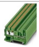
Feed-through terminal block, Connection method: Push-in / plug connection, Number of positions: 1, Cross section: 0.14 mm<sup>2</sup> - 4 mm<sup>2</sup>, AWG: 26 - 12, Width: 5.2 mm, Color: green, Mounting type: NS 35/7,5, NS 35/15
