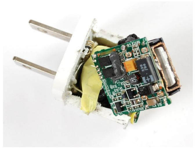
Taking it apart, desoldering the 4 data line resistors and measuring them on our multimeter, we found the following as shown in the schematic:
