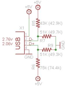
The four resistors create a voltage at each of the data lines that's not 3.3V but rather 2.8 and 2.0 (or so) volts. The problem is that when you do this, the iPhone starts to draw as
