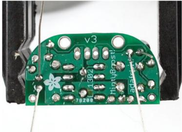
Solder in the two capacitors then clip the wires.
