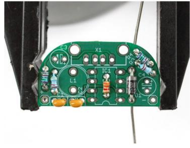
make sure energy is transfered in only one direction-from the batteries to the USB port. Diodes have a special property that current can only pass thru them in one direction. That means that it is important to make sure that they are not inserted in backwards. Examine the diode and find the end with a white stripe. This stripe should match up with the silkscreen image, which also has a stripe on one end. In this image, it is towards the top.
