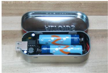
You're done! Remember that because the boost chip uses virtually no power, you dont have to remove the batteries to turn off the MintyBoost. Just plug and unplug devices whenever you want.
