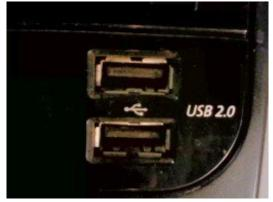
Every computer has a USB connector on it, and all the connectors are the same, with 4 pins. One pin is Ground, two pins are Data (D+ and D-) and the last pin is 5V power. The Ground and 5V pins are used to provide power to whatever is plugged in - keyboard, mouse, USB key, etc. The two data lines are used to transfer information back and forth - what keys are pressed, saving files to the USB drive, etc.
