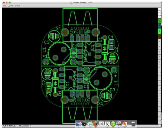
I always check the boards with <a href="www.freedfm.com">www.freedfm.com</a> (http://adafru.it/c4j) before I ship them off to be made. I used 4pcb.com so it's the same company but even if you don't go with 4pcb.com as your PCB manufacturer, it's a neat service.
