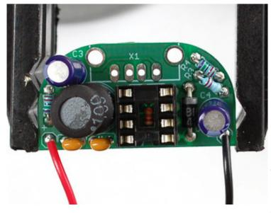
Next, solder in the 2xAA battery holder. The red wire goes to the hole marked + and the black wire goes to the hole marked -.
