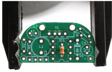
The first part we will place is the resistor **R5** - this is a small oval tan thing with two wires (leads) and color stripes. The stripes are orange orange red which indicates a 3.3K resistor. This resistor is used to improve the high current capability of the boost converter chip and is a new addition to the mintyboost. The resistor goes right in the middle, over the silkscreen text that says **R5**.
