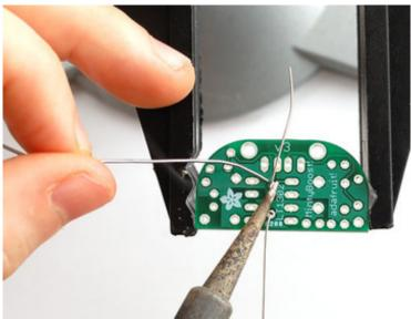
degrees. Then poke the end of the solder so that it flows into the hole and forms a solder joint.
