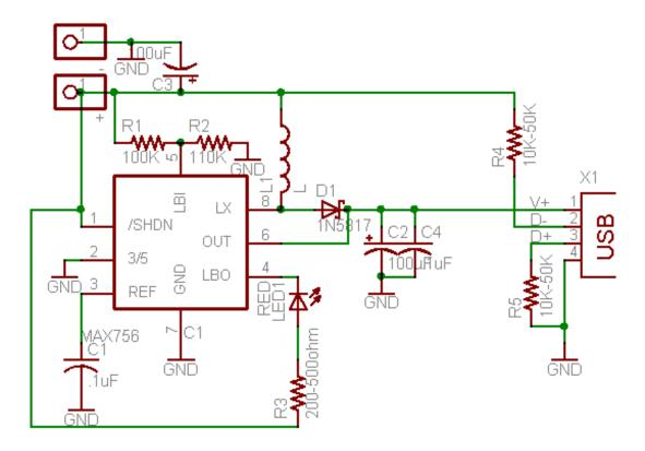
LED1, R1, R2 and R3 are optional, not included in the kit, and should be installed only if the user wants the "Low Battery Indication" function. Check the MAX756 datasheet for information on how to pick R1 and R2.
