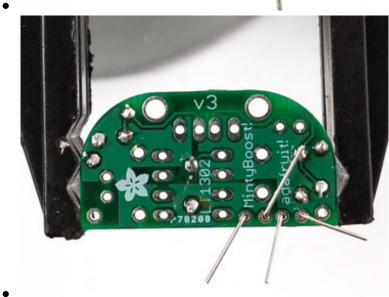
The next type of part we'll place is the ceramic capacitor. These are parts **C1** and **C2**. Ceramic capacitors have a nice property that they are symmetric/non-polarized. That means they can go in 'either way'. Place the capacitor so that the 2 legs (leads) slide thru the two metal holes in the PCB (pads). The capacitor will sit flat against the PCB.
