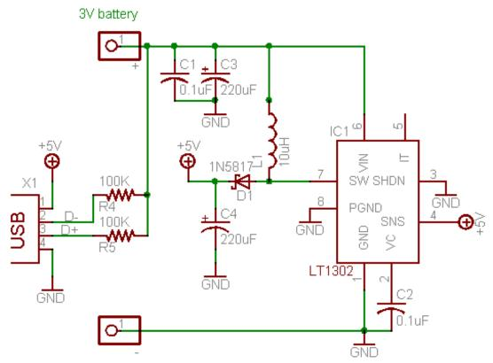
Smartphones started coming out and becoming popular, and devices with massive batteries, which meant that charging at 100mA was a no go. The mintyboost was then upgraded to the <u>LT1302</u> (http://adafru.it/c3U), a more expensive chip but one with a nice 500mA output ability!
