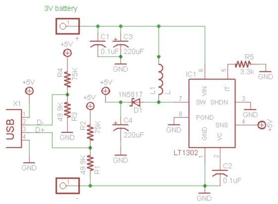
To improve compatibility with the latest smartphones and Apple devices, the charging protocol was reverse engineered so that the Mintyboost would be more universal. The pullup/down pins were also changed a full resistive divider which made it work with LiPoly batteries and Apple devices (http://adafru.it/c3k). Still uses a LT1302 chip.
