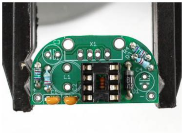
in so that the notch in the edge of the socket matches up with the notch in the silkscreen image of the socket. In this image it's near the bottom. If you mess this up, dont try to desolder the socket, instead just keep going and remember that it is upside down later when it's time to install the chip.
