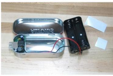
Once you're happy, remove the electronics and put the doublesided sticky foamtape on both the circuit board and the battery holder.
