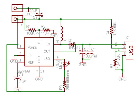
After a few months it became clear that some devices especially Apple music players, needed pullup/down resistors, so a new version that could fit 1 pullup and 1 pulldown was designed. This version still used the MAX756 (http://adafru.it/c3T).
