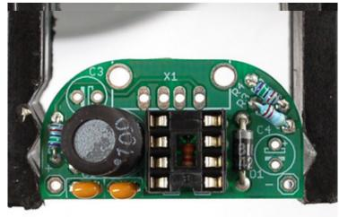
Next is the power inductor **L1**. This component is used by the DC/DC converter chip to store and convert power from low voltages to high. Inductors are just a coil of wire so they have no polarity and can be placed either way.
