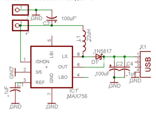
All these parts must fit into the space left over from the battery pack. I make EagleCAD library parts for the inductor and chip (the rest are already there) and lay out the board. I'm not going to detail making library parts in eagle or pcb layout, others have done so already. Use whichever software you want, I like Eagle because there's a free version available for download if you're just making small PCBs.
