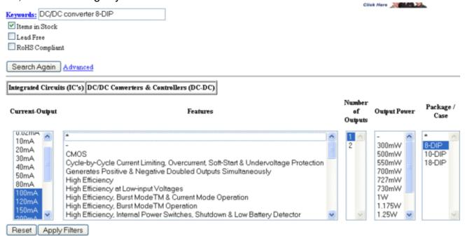
I then select 1 output, 8-DIP (to differentiate between 18-DIP) and select all the current-outputs >=100mA and apply the filter. There's still about 40 options. So then I select the all voltage input ranges that start with 2V or less. Also I select all the Adjustable, and 5V-inclusive output voltage options.
