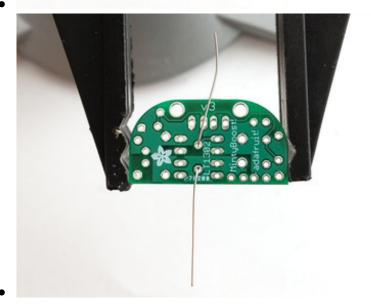
Now you'll solder! Place the flat of the soldering iron tip against the silver ring (pad) and one of the wires of the resistor (lead) at the same time for 2 seconds. This will heat them both up to 600-700
