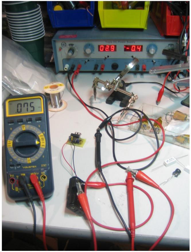
That means that the self-discharge rate is ~2000mAh / 0.1mA = 20,000 hours, more than 2
