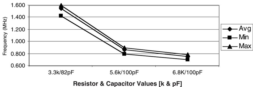
Figure 7: Internal Oscillator Frequency
