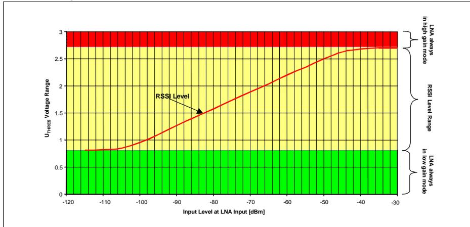
**Figure 4 RSSI Level and Permissible AGC Threshold Levels**
