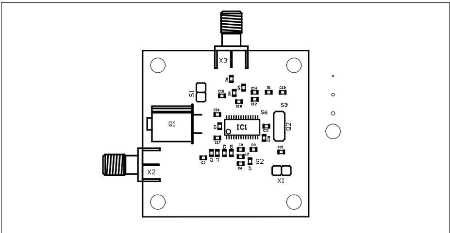
Figure 18 Component Placement on the Evaluation Board
