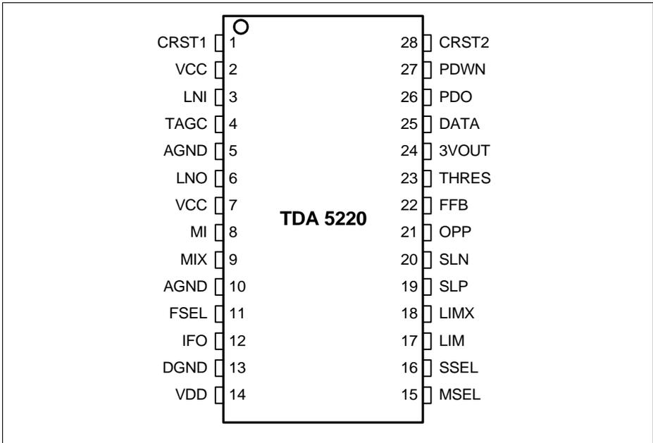
Figure 1 Pin Configuration
