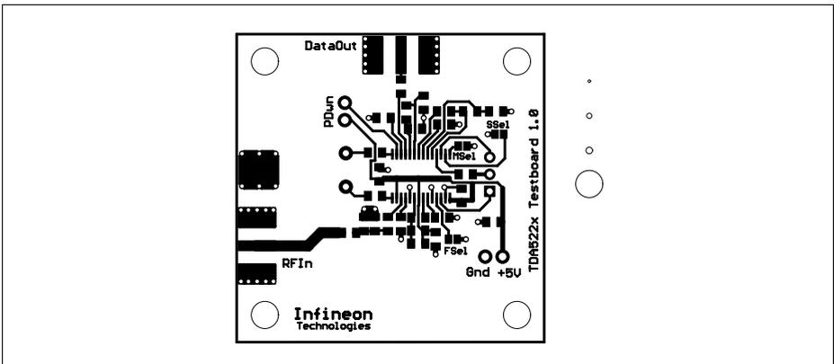
Figure 16 Top Side of the Evaluation Board
