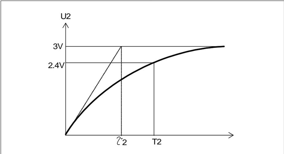
**Figure 13 Voltage appearing on C18 during precharging process**
