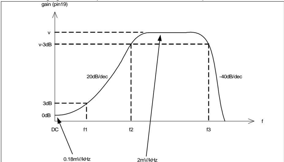
**Figure 10 Frequency characteristic in case of FSK mode**
