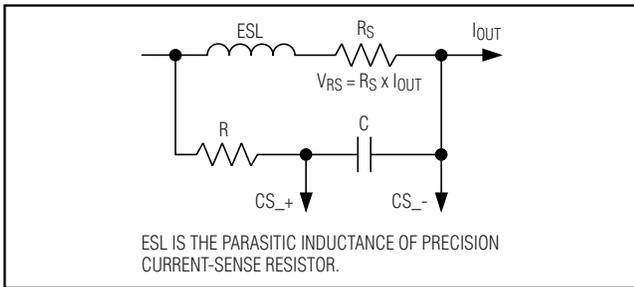
Figure 2. Current-Sense Resistor
