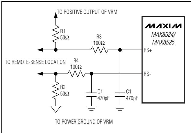
Figure 3. Recommended Filtering for Output-Voltage Remote Sensing
