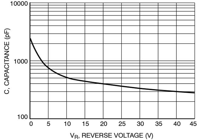
Figure 7. Typical Capacitance
