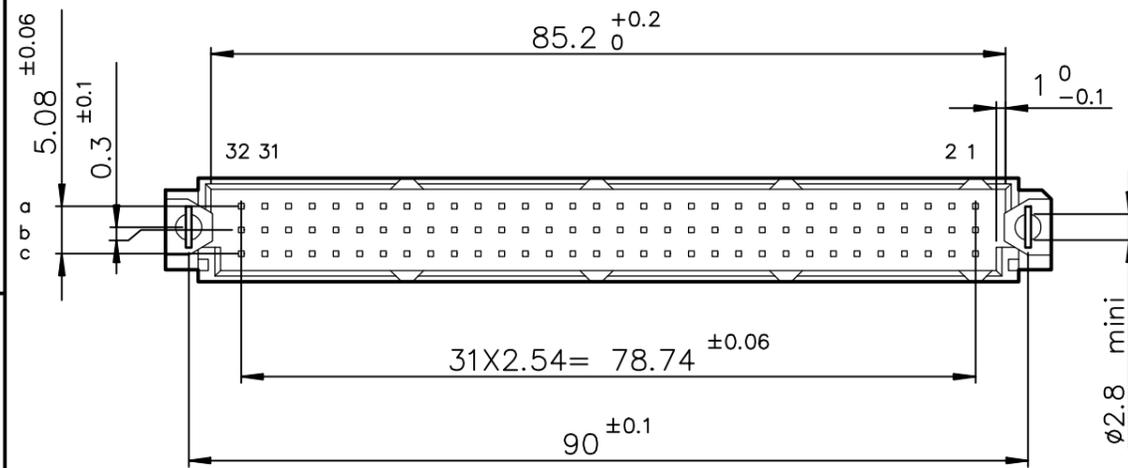
P.C. CARD DRILLING (Component side view)
