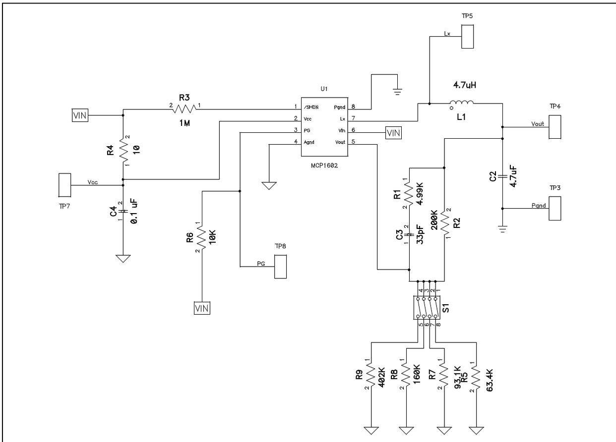
**FIGURE 1-1:** MCP1602 Typical Applications With Adjustable Output Voltage.
