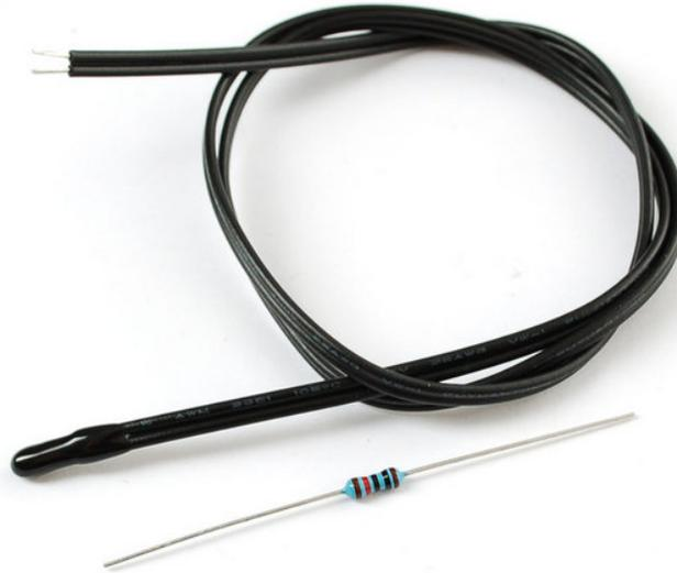
There are two kinds of thermistors, NTC (negative temperature coefficient) and PTC (positive temperature coefficient). In general, you will see NTC sensors used for temperature measurement. PTC's are often used as resettable fuses - an increase in temperature increases the resistance which means that as more current passes thru them, they heat up and 'choke back' the current, quite handy for protecting circuits!
