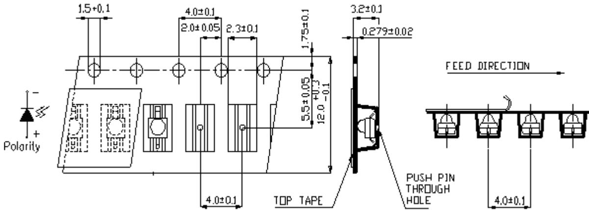
Note: The tolerances unless mentioned are ±0.1, unit=mm.
