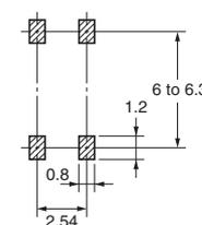
\* The external dimensions are different from those of the standard SOP 4-pin, but the mounting pad dimensions are the same.
