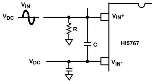
FIGURE 19. DC COUPLED SINGLE ENDED INPUT
