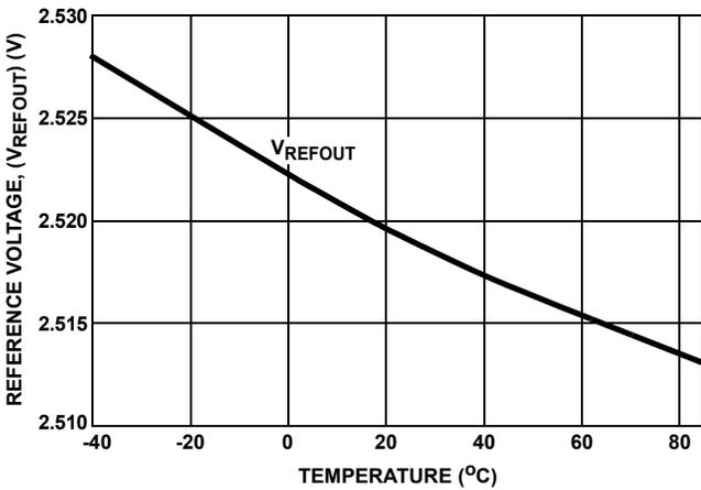
FIGURE 10. INTERNAL REFERENCE VOLTAGE (VREFOUT) vs TEMPERATURE
