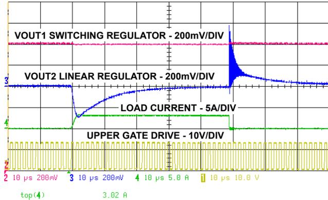
FIGURE 5. LINEAR REGULATOR RESPONSE TO 3A TRANSIENT LOADING
