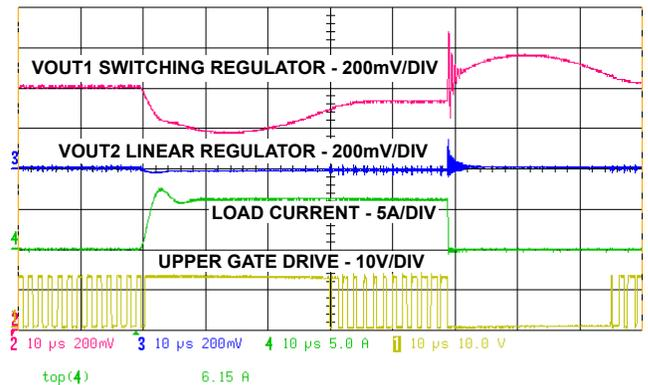
FIGURE 4. SWITCHING REGULATOR RESPONSE TO 6A TRANSIENT LOADING
