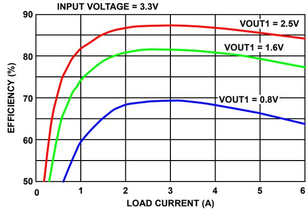
FIGURE 7. EFFICIENCY vs LOAD CURRENT FOR 3 OUTPUT VOLTAGES
