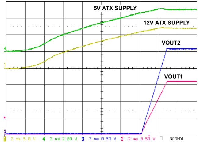
FIGURE 3. SOFT-START WAVEFORMS
