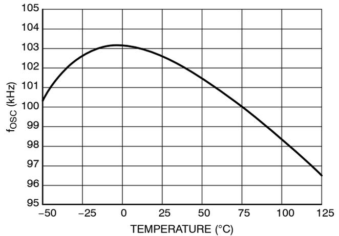
Figure 14. Oscillator Frequency  $f_{\text{osc}}$  for the 100 kHz version
