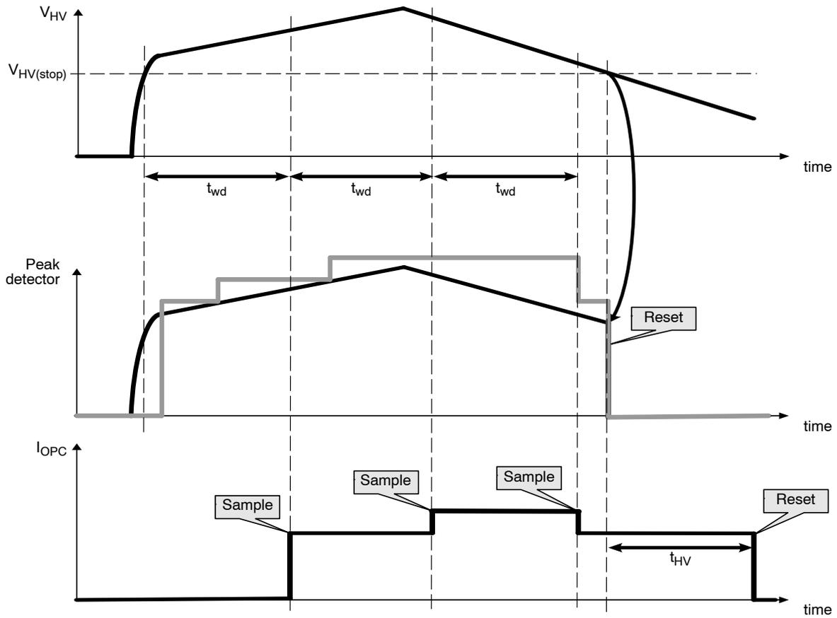
**Figure 42. Overpower Compensation**
