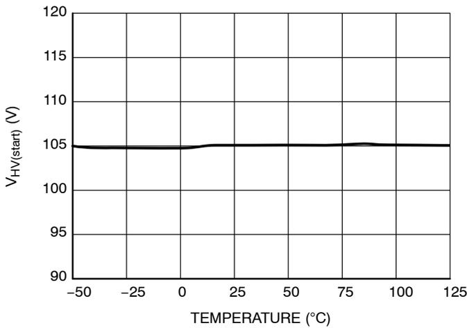
Figure 5. Brown-out Device Start Threshold
