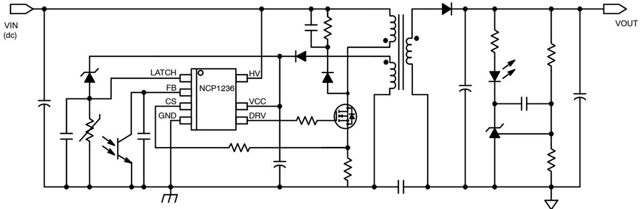
Figure 1. Flyback Converter Application Using the NCP1236
