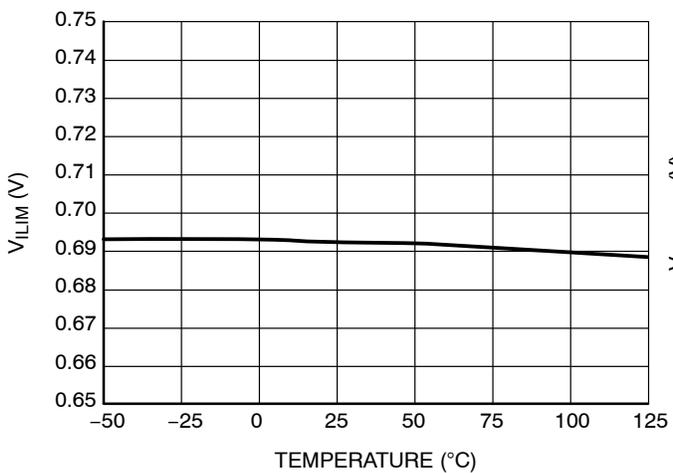
Figure 7. Maximum Internal Current Setpoint
