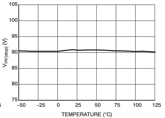
Figure 6. Brown-out Device Stop Threshold
