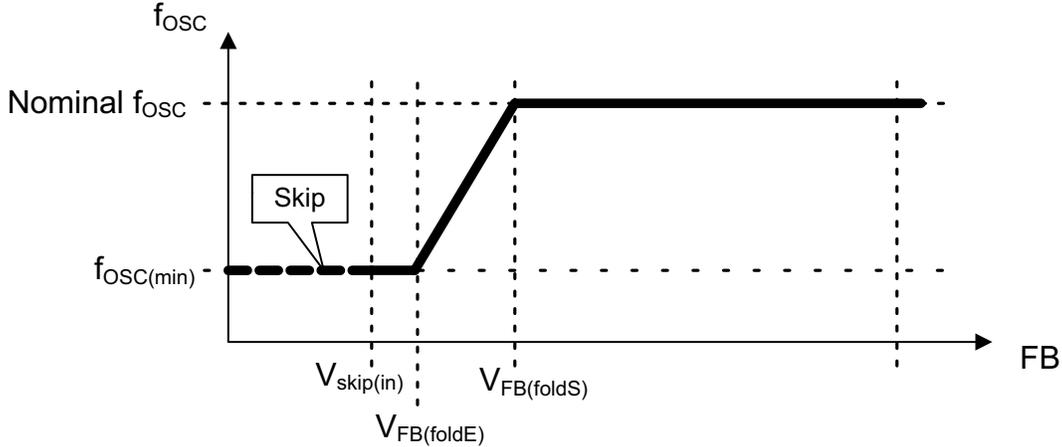
Figure 47. Frequency Foldback when the FB Voltage Decreases
