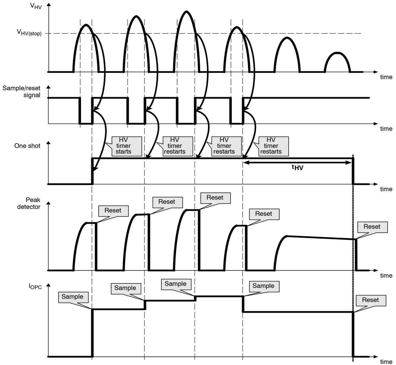
Figure 41. Overpower Compensation
