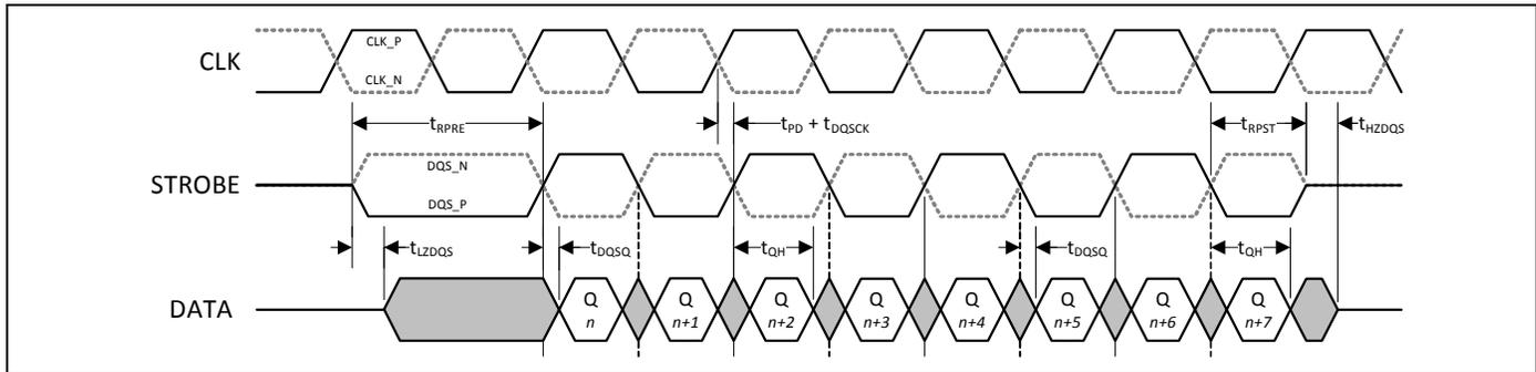
**Figure 20. DDR3 DRAM Write Timing**
