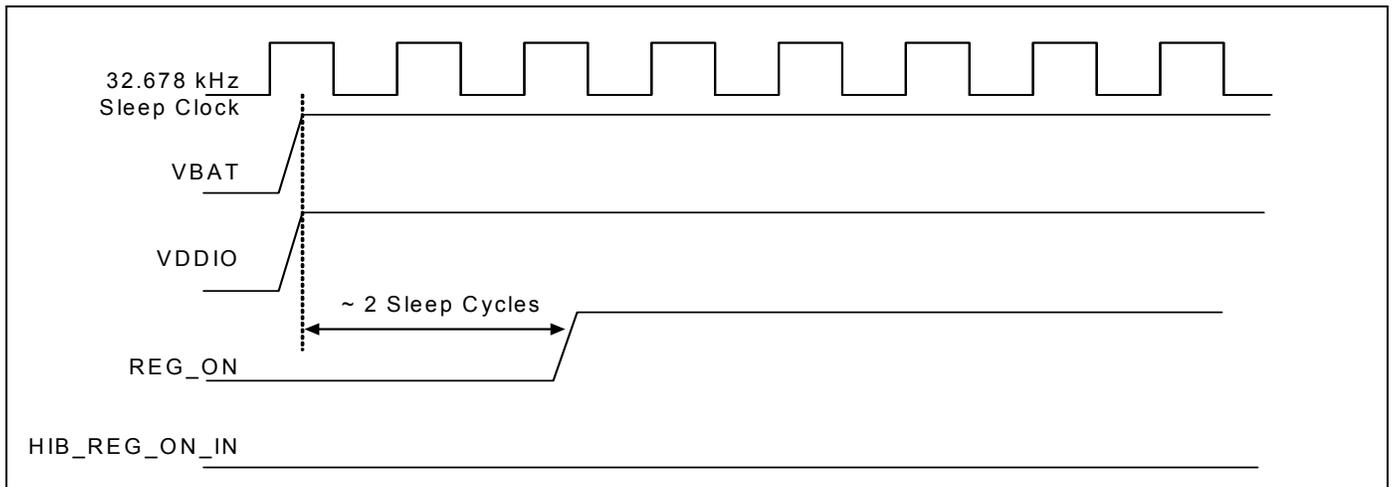
**Figure 44. HIB\_REG\_ON\_IN = High, HIB\_REG\_ON\_OUT Connected to REG\_ON**
