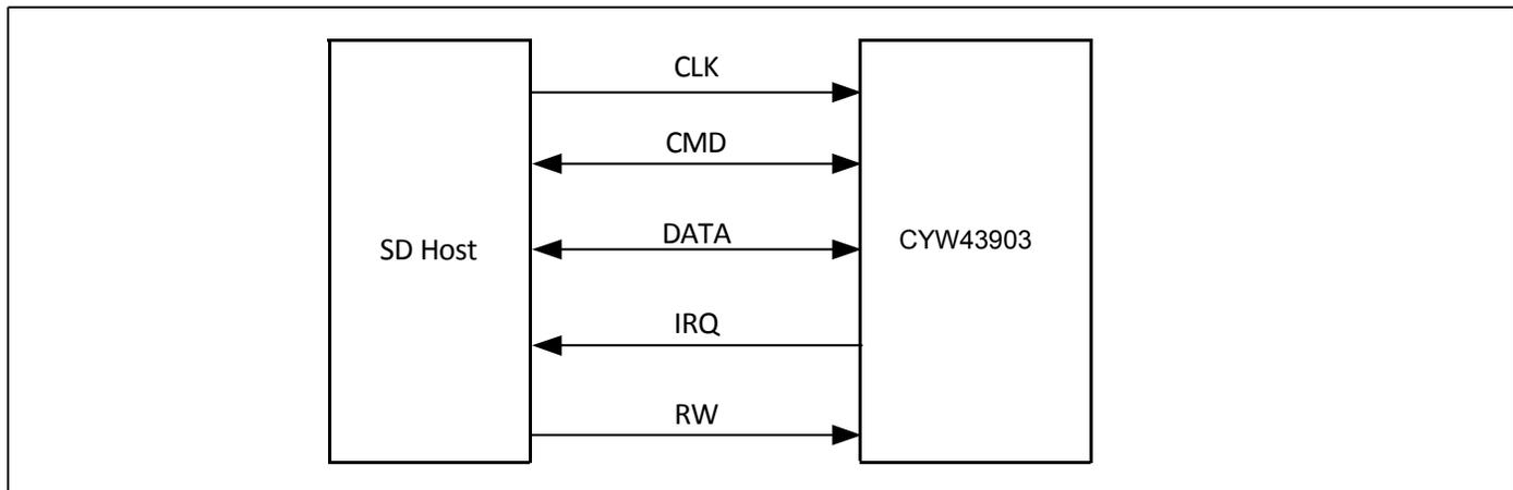
**Note:** Per Section 6 of the SDIO specification, pull-ups in the 10 kΩ to 100 kΩ range are required on the four data (DATA) lines and the command (CMD) line. This requirement must be met during all operating states either through the use of external pull-up resistors or through proper programming of the SDIO host's internal pull-ups
