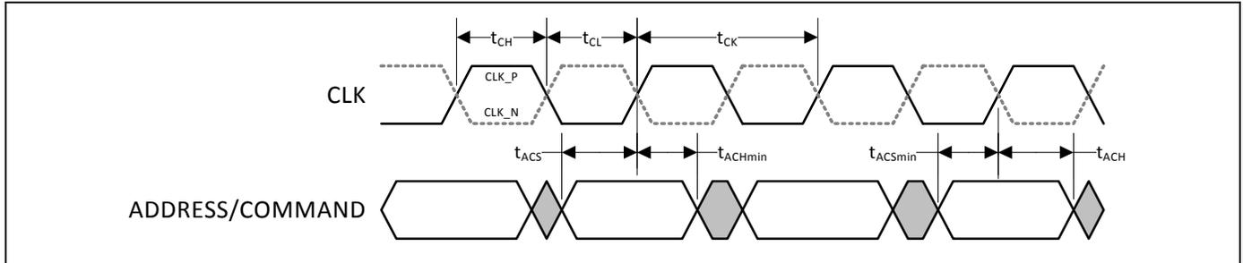
**Figure 19. DDR3 DRAM Read Timing**
