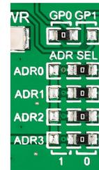
The board features a set of four onboard jumpers [zero ohm resistors] for specifying a unique address for the sensor. A separate jumper lets you select the sensor's output between GP01 and GP0 pins.
