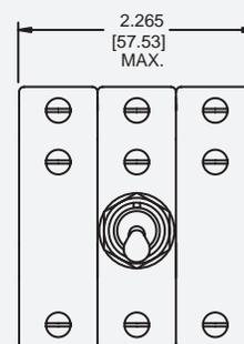
Panel Mounting Details: Tolerance  $\pm 0.005$  [.13] Unless noted.
