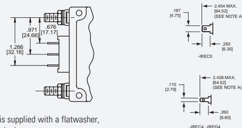
Note: Each outer terminal is supplied with a flatwasher, tooth lockwasher and a hex nut.
