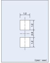
The recommended thickness of the screen mask for soldering is more than  $150\,\mu\text{m}.$  The hole size of the screen mask should be same as the recommended land pattern or smaller.
