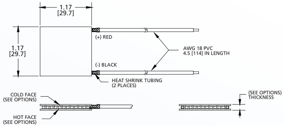
Ceramic Material: Alumina ( $\text{Al}_2\text{O}_3$ )
