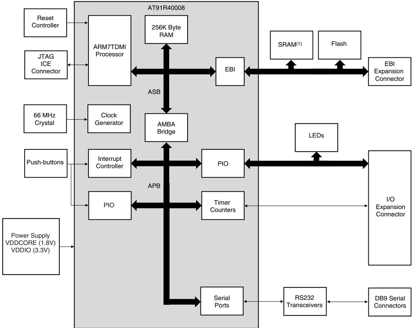
**Note:** No external SRAM is fitted on the board. See section “Memories” on page 4-1 for more details.
