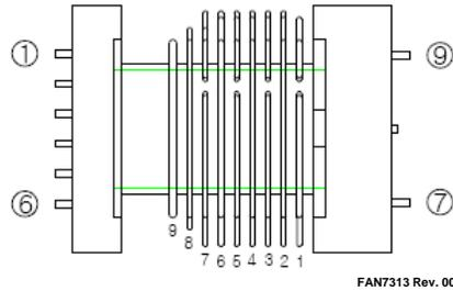
Figure 5. Transformer Schematic
