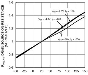
T<sub>J</sub>, JUNCTION TEMPERATURE (°C) Figure 6 On-Resistance Variation with Temperature
