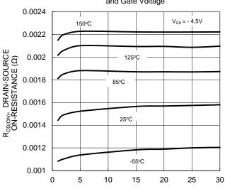
${\rm I_D},\,{\rm DRAIN\,\,CURRENT(A)}$  Figure 5 Typical On-Resistance vs. Drain Current and Temperature
