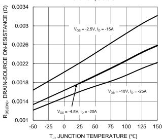
Figure 7 On-Resistance Variation with Temperature
