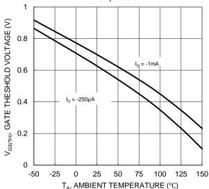
$\rm T_A, \, AMBIENT \, TEMPERATURE \, (^{\circ}C)$  Figure 8 Gate Theshold Variation vs Ambient Temperature
