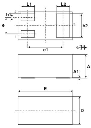
*Note: Product marking may be rotated by 90° for assembly plant differentiation. In no case should this product marking be used to orient the component for its placement on a PCB. Only pin 1 mark is to be used for this purpose.*
