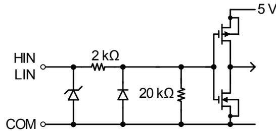
$\overline{FO}$  Internal Equivalent Circuit
