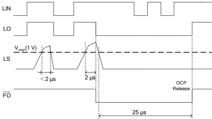
OCL Protection Circuit Timing (OCL and SD connected)
