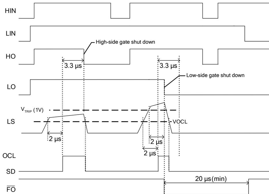
TSD Protection Circuit Timing
