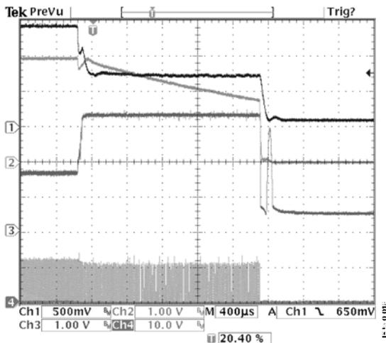
Figure 7. Overcurrent Latch-Off Waveforms
