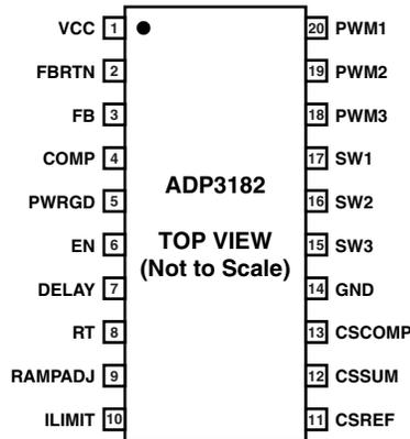
Figure 3. Pin Configuration
