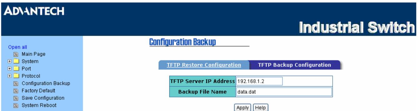
Figure 3.1-35 TFTP Backup Configuration
