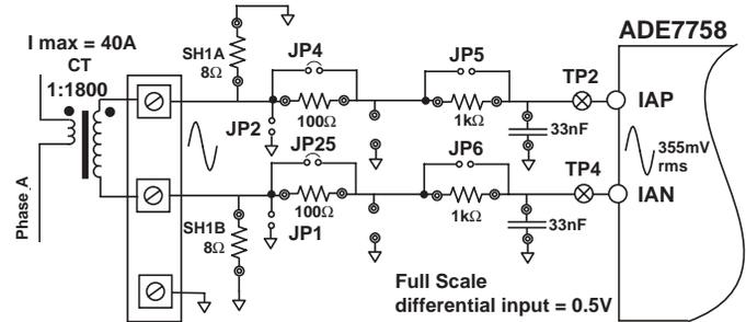
Figure 2 — CT connection to Current Channel
