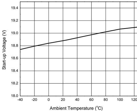
**Minimal Operating Voltage vs. Ambient Temperature**
