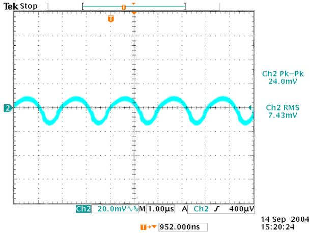
Figure 13: Output ripple & noise at 12Vin, 3.3V/4A out
