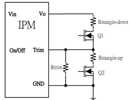
**Figure 33:** Circuit configuration for output voltage margining
