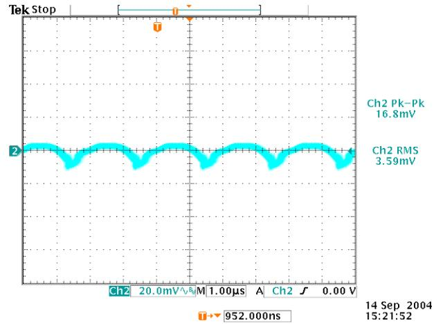
Figure 10: Output ripple & noise at 12Vin, 1.5V/4A out
