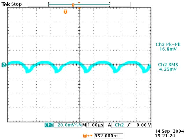
Figure 11: Output ripple & noise at 12Vin, 1.8V/4A out
