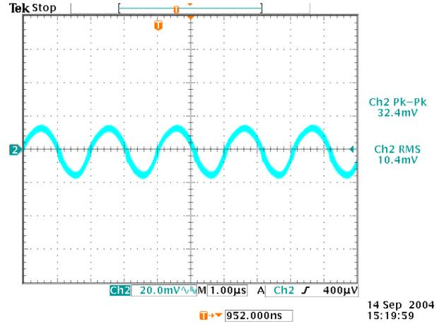
Figure 14: Output ripple & noise at 12Vin, 5.0V/4A out
