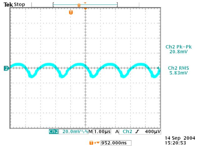
Figure 12: Output ripple & noise at 12Vin, 2.5V/4A out
