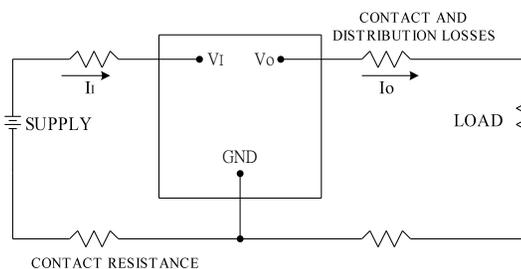
**Figure 27:** Output voltage and efficiency measurement test setup
