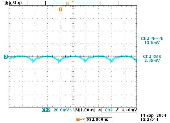
Figure 8: Output ripple & noise at 12Vin, 0.9V/4A out
