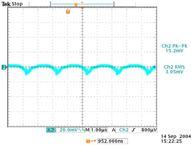
Figure 9: Output ripple & noise at 12Vin, 1.2V/4A out
