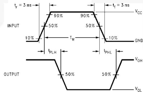
Figure 6. AC Waveforms
