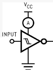
Figure 7. I<sub>CCD</sub> Test Circuit
