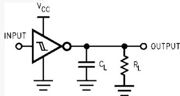
Figure 5. AC Test Circuit
