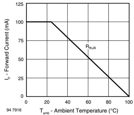
Fig. 2 - Forward Current vs. Ambient Temperature
