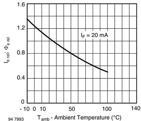
Fig. 8 - Relative Radiant Intensity/Power vs. Ambient Temperature
