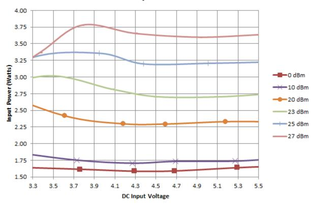
Note: Power consumption is defined for operation into a 17 dB return loss load (VSWR of 1.33) or better. Power consumption may increase, up to 4 W, during operation into return losses worse than 17 dB and high ambient temperatures. Power consumption will also vary based on which of the <a href="Supported Regions">Supported Regions</a> is in use.
