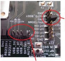
The SHUTDOWN line will turn off the Nano module if connected to GND. For normal operation, do not connect SHUTDOWN to GND.
