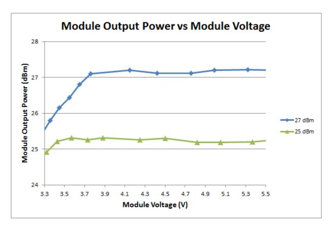
The power drawn by the module is fairly constant, rising slightly as the DC Input Voltage is lowered. Once the 1A input current limit is reached, the input power appears to
