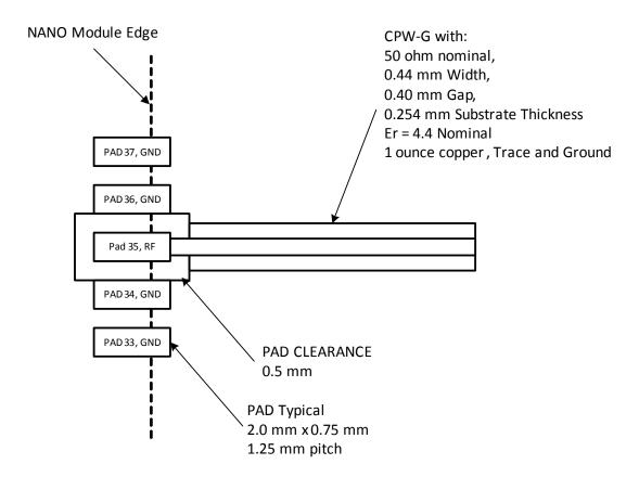
The area beneath the module should be kept clear of traces and copper.
