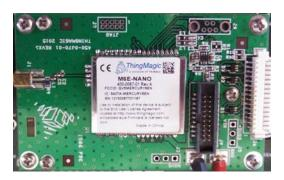
ThingMagic has created a Carrier Board for the ThingMagic Nano module, as an example of a host board for this module and to create an assembly that is compatible with the standard Development Kit main board. It has the size and dimensions of the M6e module (69 mm x 43 mm), and uses the same connector for power and control (Molex 53261-1571 - 1.25mm pin centers, 1 amp per pin rating. which mates with Molex housing p/n 51021-1500 with crimps p/n 63811-0300).
