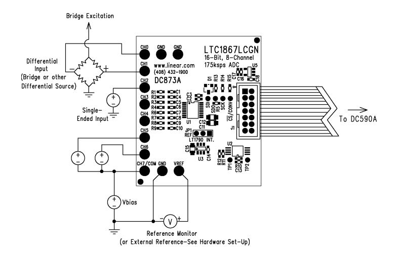
Figure 1. Connection Diagram
