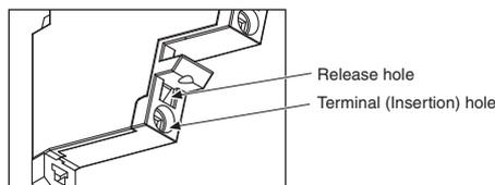
**Connecting Wires with Ferrules and Solid Wires**
