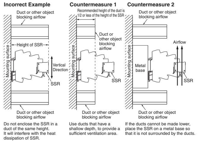
Do not enclose the SSR in a duct of the same height. It will interfere with the heat dissipation of SSR.
