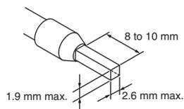
3. If you use AWG24 to AWG22 (0.25 to 0.34 mm<sup>2</sup>) wires, UL certification will not apply.
