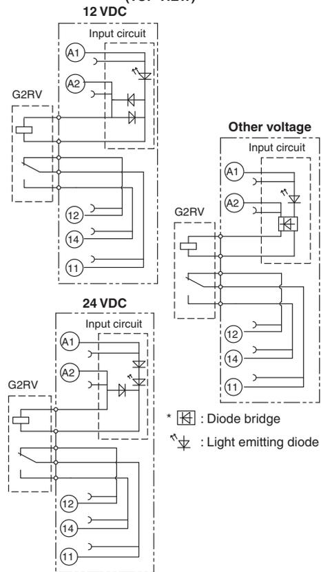
**Models with latching lever (with test switch)**
