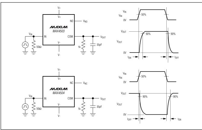
Figure 1. Switching Times
