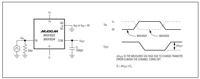
Figure 2. Charge Injection
