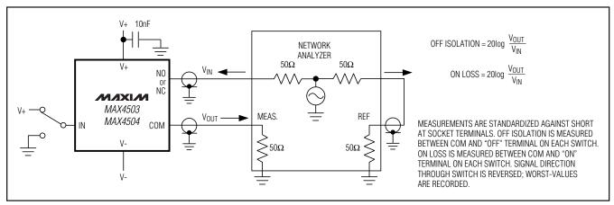
Figure 3. Off Isolation and On Loss
