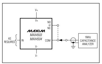
Figure 4. NO, NC, and COM Capacitance
