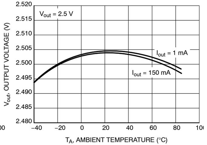
Figure 4. Output Voltage vs. Temperature
