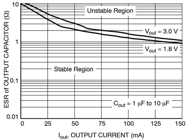
Figure 23. Output Capacitor ESR vs. Output Current
