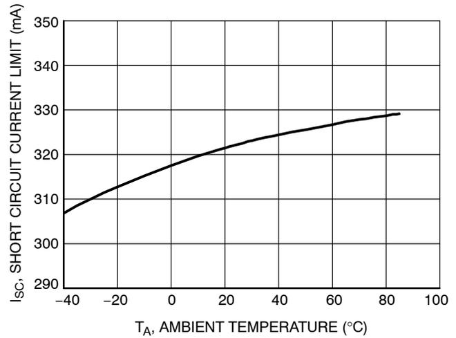
Figure 17. Short Circuit Current vs. Temperature
