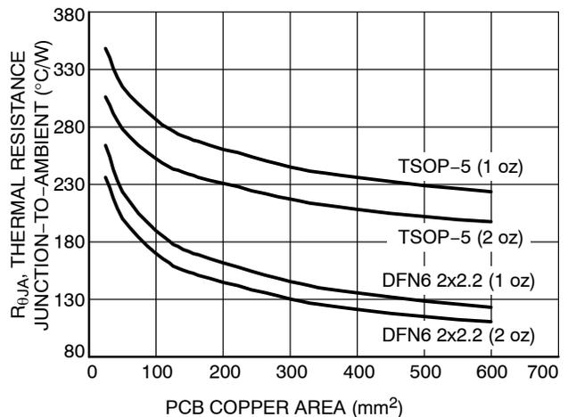
**Figure 24.  $R_{\theta JA}$  vs. PCB Copper Area**
