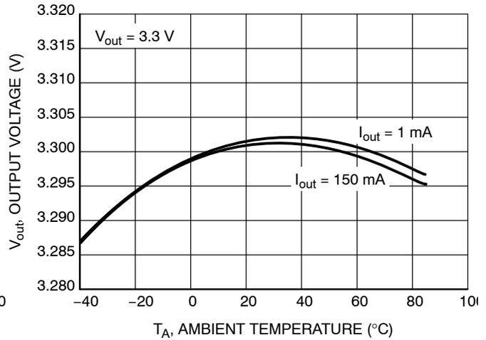
Figure 8. Output Voltage vs. Temperature
