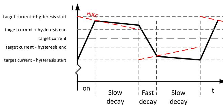
Figure 2: spreadCycle principle
