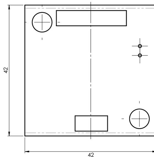
Figure 6: PD42-1270 top view mechanical dimensions
