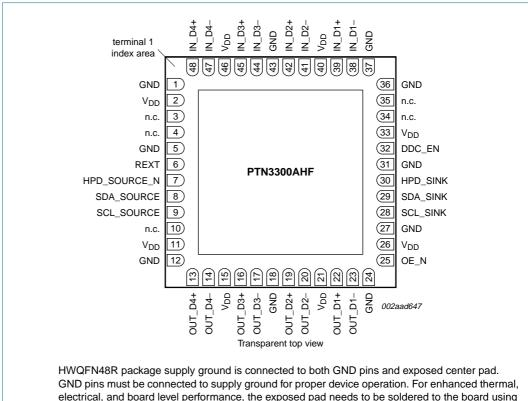
GND pins must be connected to supply ground for proper device operation. For enhanced thermal, electrical, and board level performance, the exposed pad needs to be soldered to the board using a corresponding thermal pad on the board and for proper heat conduction through the board, thermal vias need to be incorporated in the PCB in the thermal pad region.
