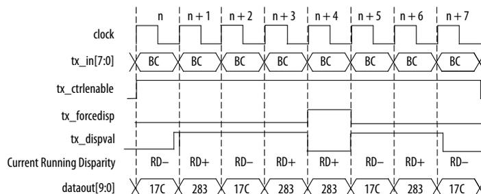
Refer to the *8B/10B Encoder Current Running Disparity Control Feature* section for more information about the 8B/10B data current running disparity control.
