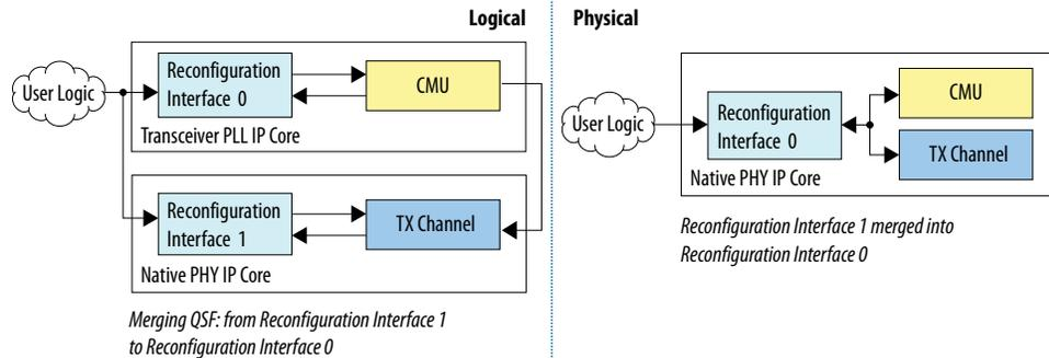
**Rules for Merging Reconfiguration Interfaces Across Multiple IP Cores**
