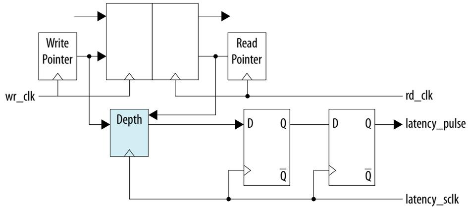
To measure the fullness of the FIFO, you must run your sampling clock at a rate that is not equal to the parallel clock. For example,  $parallel\_clock * (128/127)$  or  $parallel\_clock * (64/127)$  so that the sampling clock sweeps various phase relationships relative to the parallel clock. You must determine via a simple counter how often the resulting pulse is a 1 versus a 0. The following sample pseudo-code describes how to accomplish this:
