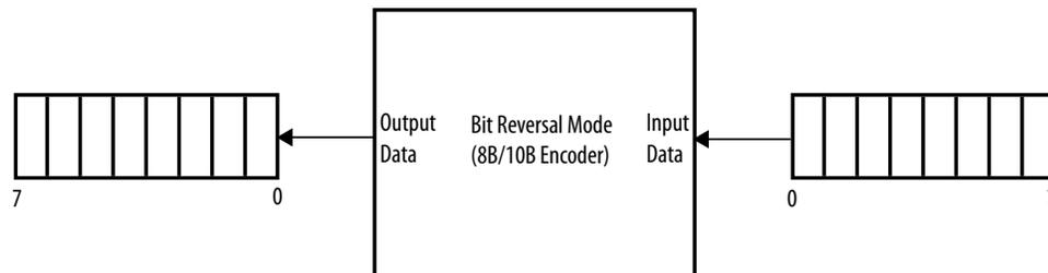
The bit reversal feature reverses the order of the bits of the input data. Bit reversal is performed at the output of the 8B/10B Encoder and is available even when the 8B/10B Encoder is disabled. For example, if the input data is 20-bits wide, bit reversal switches bit [0] with bit [19], bit [1] with bit [18] and so on.
