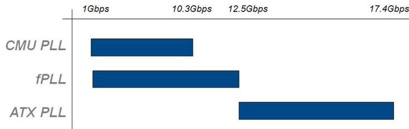
For ATX PLL VCO frequencies between 7.2 GHz and 11.4 GHz, when two ATX PLLs operate at the same VCO frequency (within 100 MHz), they must be placed 7 ATX PLLs apart (skip 6).
