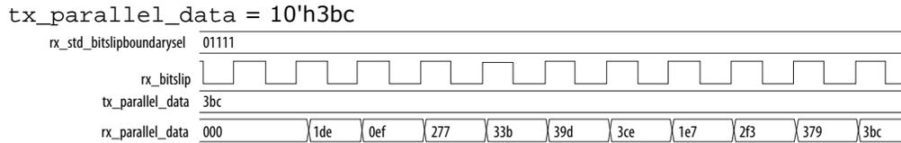
Figure 23. RX Bit Slip in 16-bit Mode
