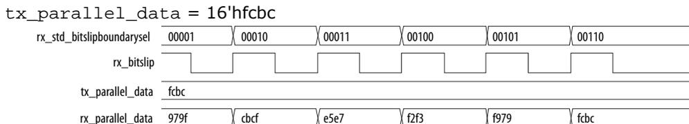
**Figure 63. RX Bit Slip in 20-bit Mode**
