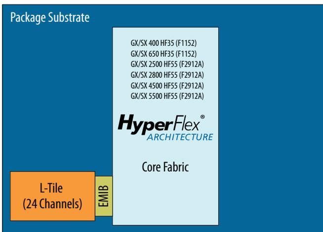
Figure 2. Stratix 10 GX/SX Device with 2 L-Tiles (48 Transceiver Channels)
