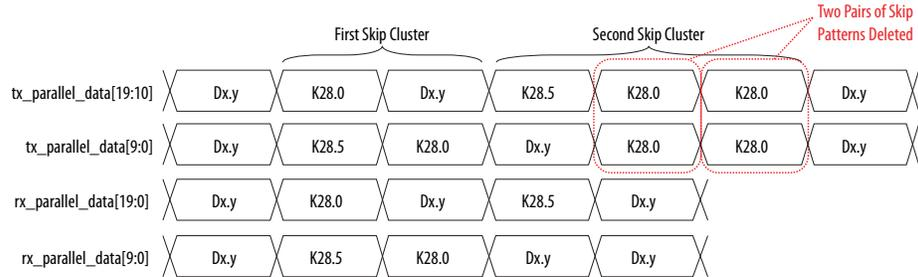
In the following figure, */K28.5/* is the control pattern and neutral disparity */K28.0/* is the skip pattern. The first skip cluster has a */K28.5/* control pattern in the LSByte and */K28.0/* skip pattern in the MSByte of a clock cycle. The rate match FIFO inserts pairs of skip patterns in this skip cluster to meet the three skip pattern insertion requirement.
