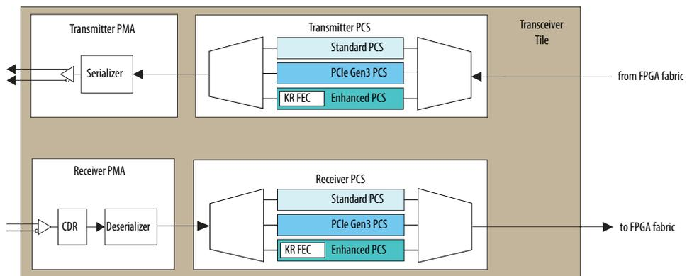
Stratix 10 GX/SX transceiver channels have three types of PCS blocks that together support continuous data rates up to 17.4 Gbps.
