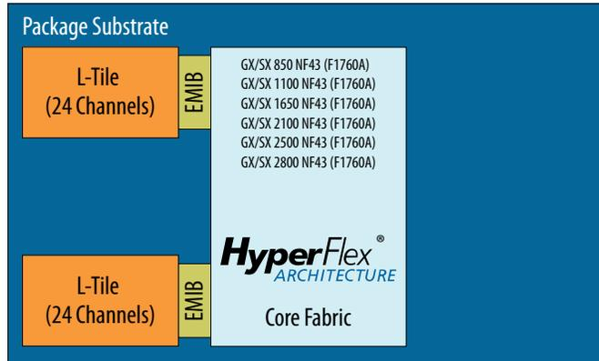
Figure 3. Stratix 10 GX/SX Device with 2 L-Tiles (48 Transceiver Channels)
