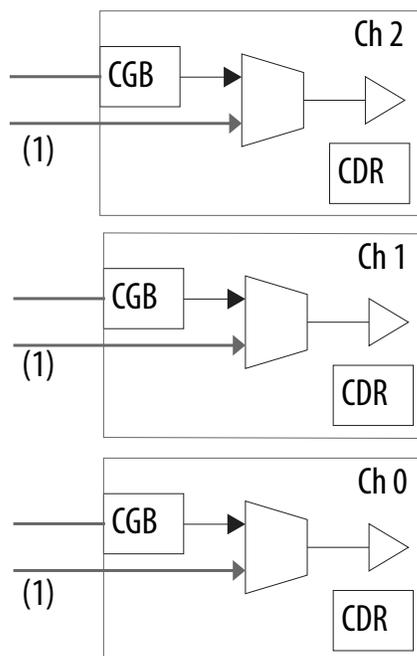
Note: (1) The local CGB is bypassed by the clock input ports in bonded mode.
