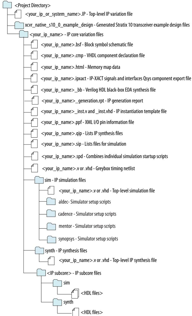
The following table describes the directories and the most important files for the parameterized Transceiver Native PHY IP core and the simulation environment. These files are in clear text.
