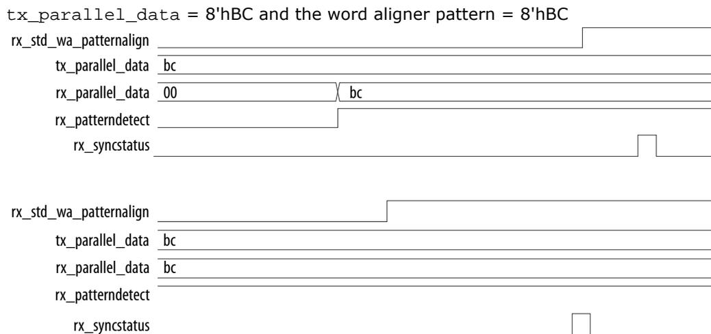
In manual alignment mode, the word alignment operation is manually controlled with the rx\_std\_wa\_patternalign input signal or the rx\_enapatternalign register. The word aligner operation is level-sensitive to rx\_enapatternalign. The word aligner asserts the rx\_syncstatus signal for one parallel clock cycle whenever it re-aligns to the new word boundary.
