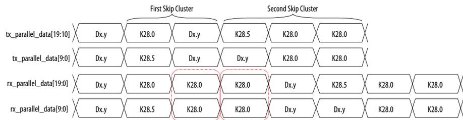
The following figure shows the deletion of the 20-bit word D7D8.
