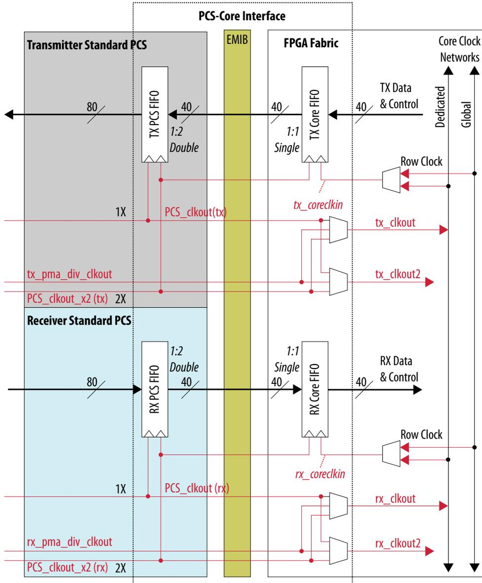
Disabling or enabling double rate transfer mode changes the parallel data mapping. Refer to the *Transceiver PHY PCS-to-Core Interface Reference Port Mapping* section for detailed data mapping information.
