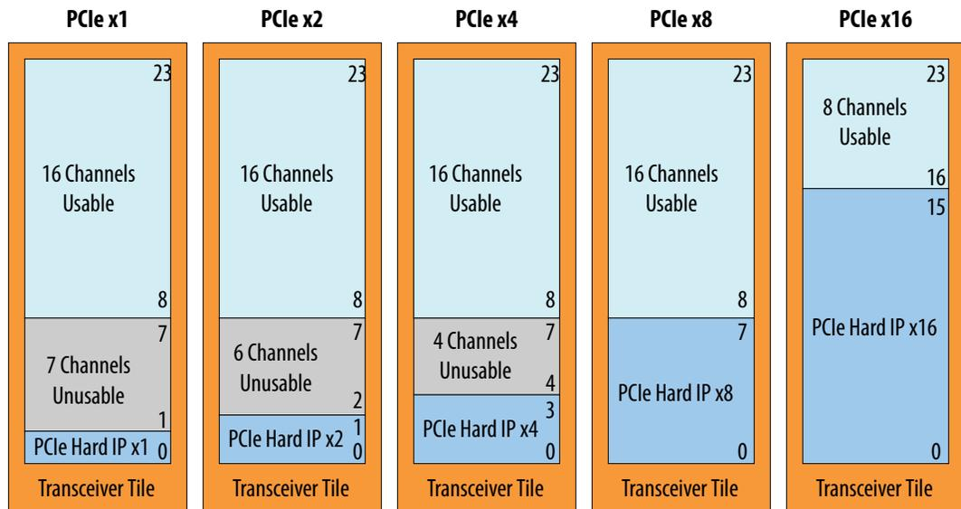
The table below maps all transceiver channels to PCIe Hard IP channels in available tiles.
