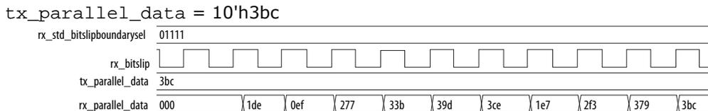
**Figure 62. RX Bit Slip in 16-bit Mode**
