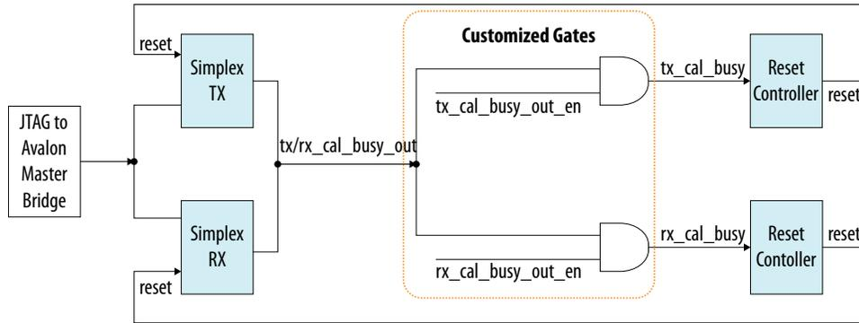
The capability register is not available for merging a Simplex TX and a Simplex RX signal into the same physical channel. The tx\_cal\_busy\_out and rx\_cal\_busy\_out signals share the same port. So, you should build customized gating logic to separate them.
