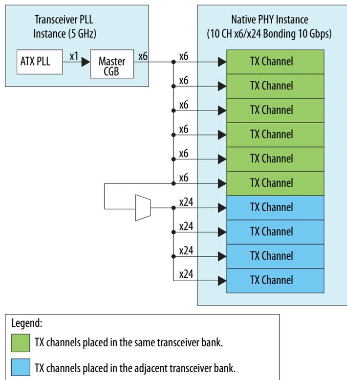
**Note:** Although the above diagram looks similar to the 10-channel non-bonded configuration example, the clock input ports on the transceiver channels bypass the local CGB in x6/x24 bonding configuration. This internal connection is taken care of when the **Native PHY channel bonding mode** is set to **Bonded**.
