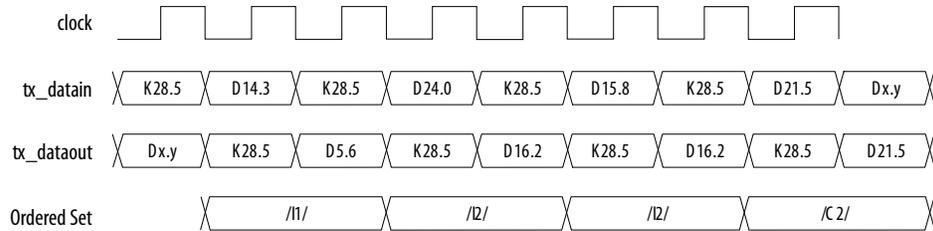
**Reset Condition for 8B/10B Encoder in GbE, GbE with IEEE 1588v2**
