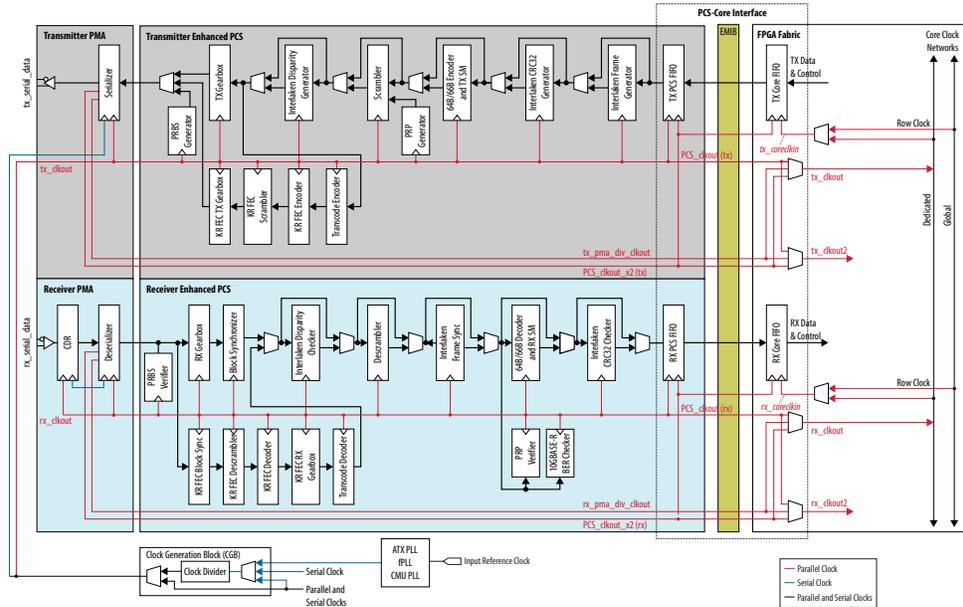
The receiver PCS forwards the following clocks to the FPGA fabric:
