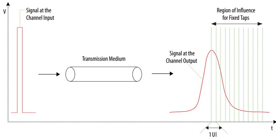
**Note:** The pulse at the output of the channel shows a long decaying tail. Frequency-dependent losses and quality degradation induces ISI.
