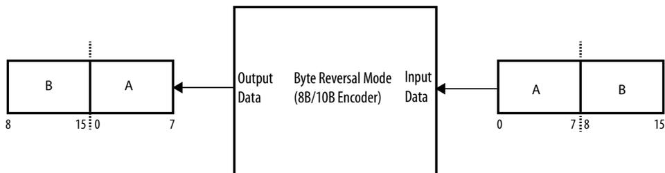
The byte reversal feature is available only when the PCS-PMA interface width is 16 bits or 20 bits. Byte reversal is performed at the output of the 8B/10B Encoder and is available even when the 8B/10B Encoder is disabled. This feature swaps the LSByte with the MSByte. For example, when the PCS-PMA interface width is 16-bits, [7:0] bits (LSByte) gets swapped with [15:8] bits (MSByte).
