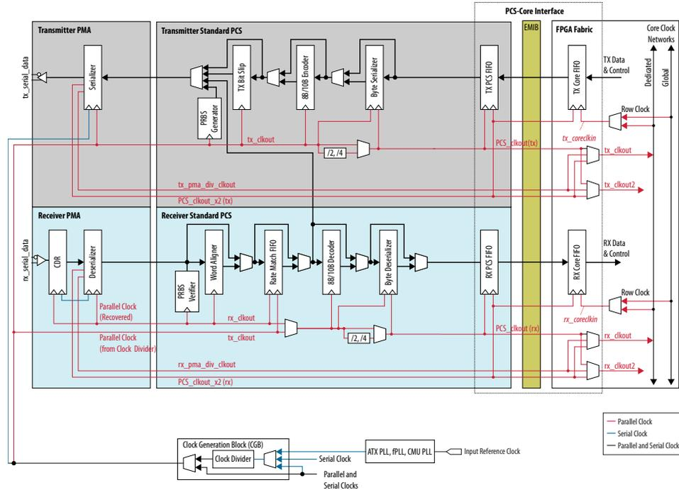
All configurations that use the Standard PCS channel must have a 0 ppm phase difference between the receiver datapath interface clock and the read side clock of the RX phase compensation FIFO.
