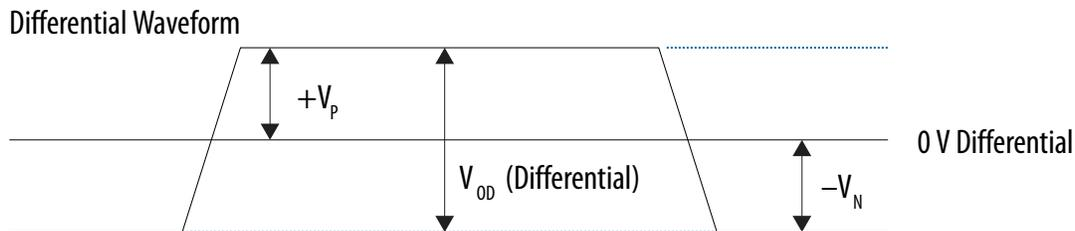
$$V_{OD} \text{ (Differential)} = V_p - V_n$$
