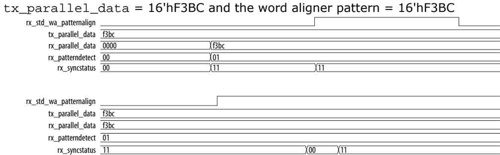
**Figure 28. Manual Mode when the PCS-PMA Interface Width is 20 Bits**
