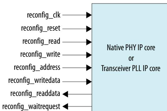
The user-accessible Avalon-MM reconfiguration interface and PreSICE Avalon-MM interface share a single internal configuration bus. This bus is arbitrated to get access to the Avalon-MM interface of the channel or PLL. Refer to the "Arbitration" section for more details about requesting access to and returning control of the internal configuration bus from PreSICE.
