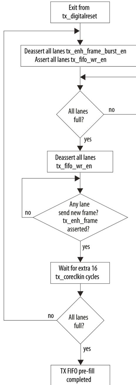
The following figure shows that after deasserting `tx_digitalreset`, TX soft bonding logic starts filling the TX FIFO until all lanes are full.
