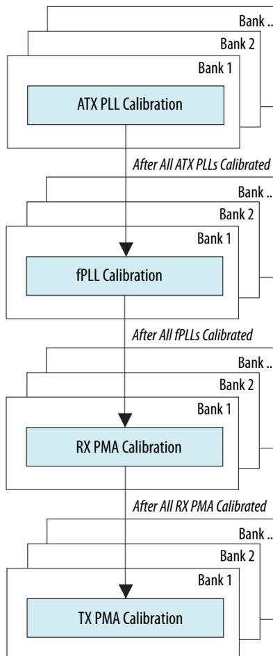
For applications using both PCIe Hard IP and non-PCIe channels, the power-up calibration sequence is:
