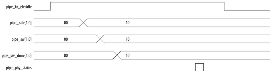
**Gen3 Transmitter Electrical Idle Generation**
