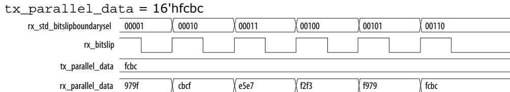
Figure 24. RX Bit Slip in 20-bit Mode
