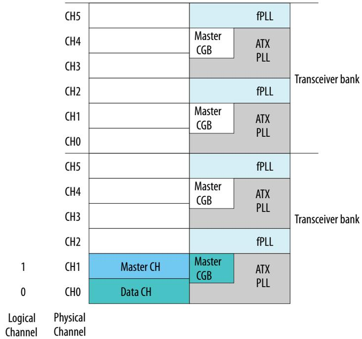
**Note:** The physical channel 0 aligns with logical channel 0. The logical PCS Master Channel 1 is specified as Physical Channel 1.
