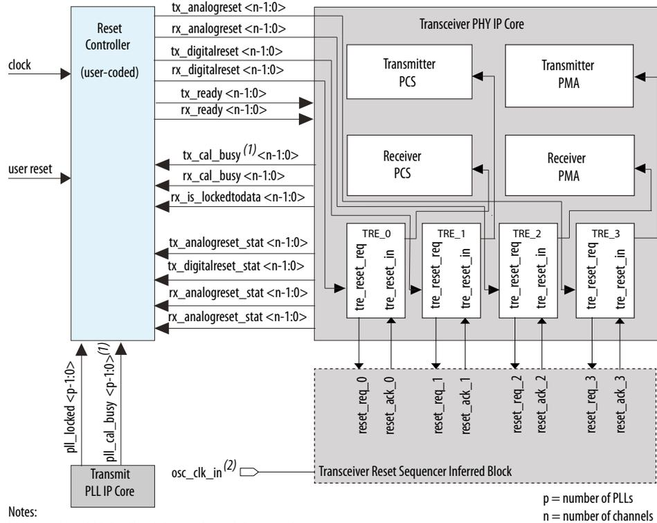
**Transceiver Reset Endpoints**—The Transceiver PHY IP core contains Transceiver Reset Endpoints (TREs). The analog and digital reset ports (both TX/RX) of the Transceiver Native PHY IP core are connected to the input of the TX TRE and RX TRE, respectively.
