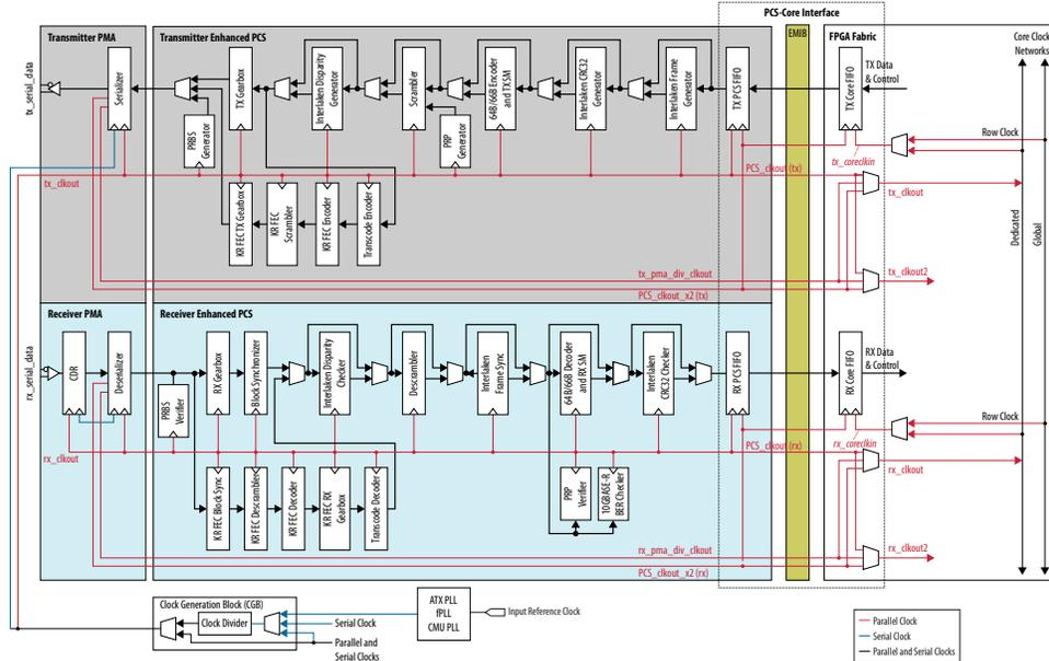
In the Enhanced PCS, the parallel clock is used by all the blocks up to the read side of the TX phase compensation FIFO. The clocks of all channels in bonded configuration are forwarded. You can pick `tx_clkout[0]` as the source for clocking their TX logic in core.
