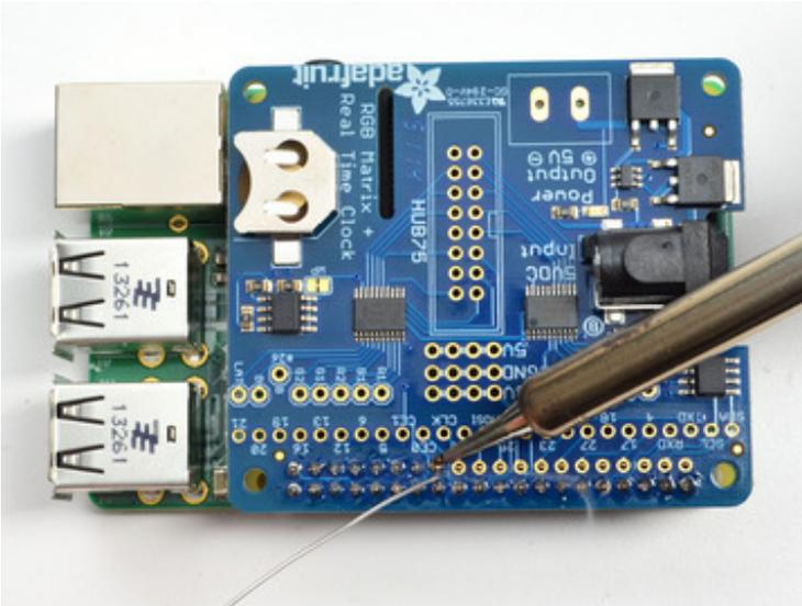
Flip the board around and solder all the connections for the other half of the 2x20 header
