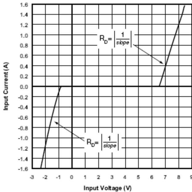
Figure 2. Typical Input VI Characteristics
