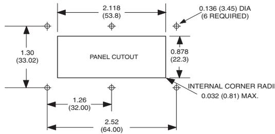
**Note:** The supplied M3 screws and washers will accommodate panel thicknesses from 0.060 to 0.090 inches (1.52 to 2.28 mm).
