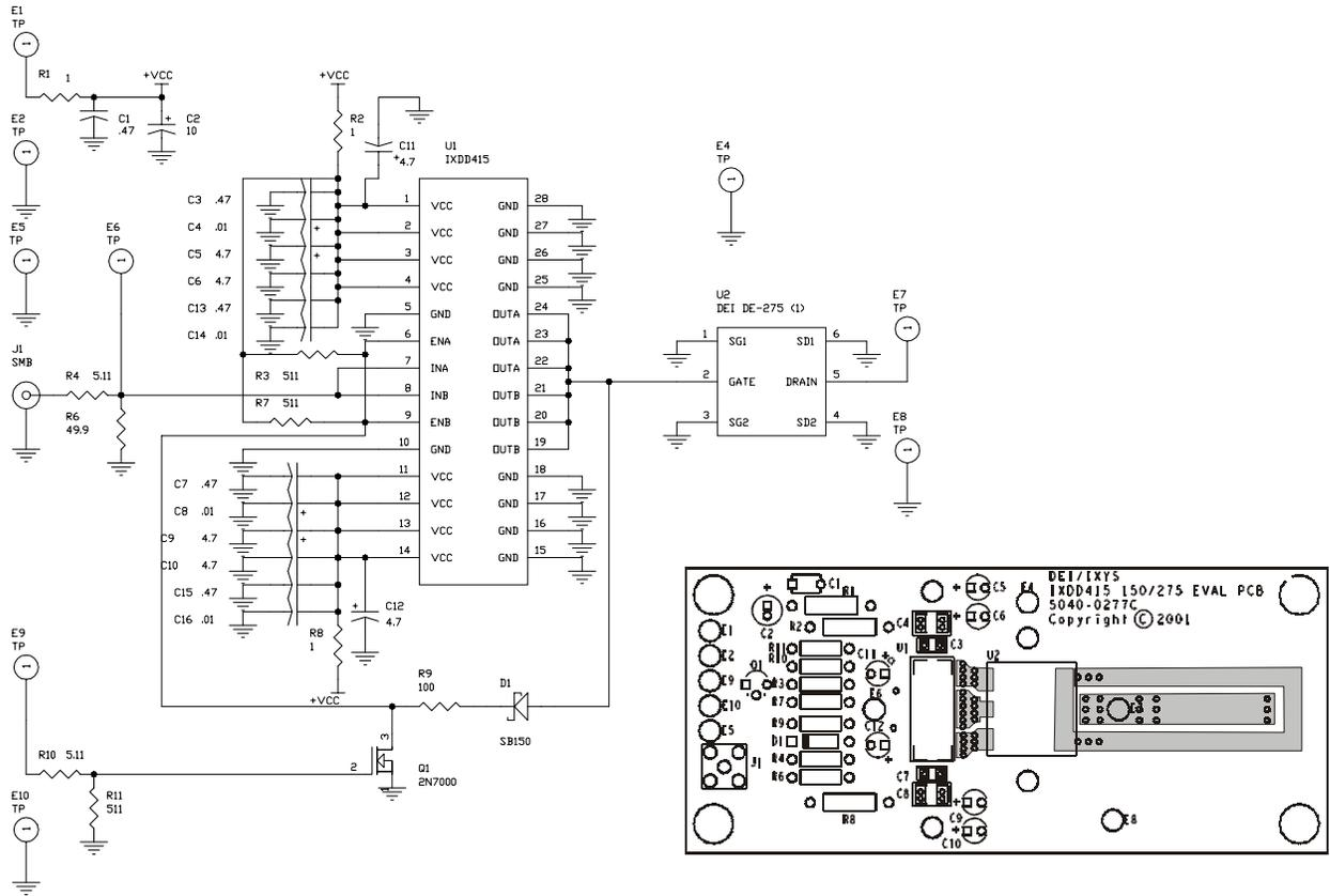
**NOTES:** 1) The schematic shows a DE275 MOSFET, however a DEI DE-150 or DE-275 package type may be installed on the EVDD415. The EVDD415 is provided without a MOSFET, so that the user can install the appropriate MOSFET for their application.
