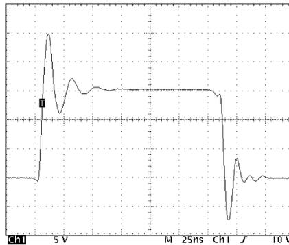
Figure 6 - EVDD415 Typical Gate Waveform
