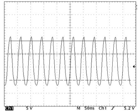
Figure 7 - EVDD415 Typical Output Waveform
