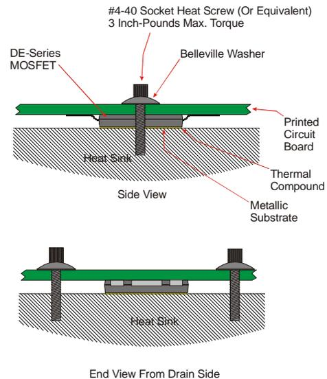
**Figure 2 - EVDD415 Side Views Showing DE-Series Power Device Installed In A High-Power Configuration<sup>(2)</sup>**
