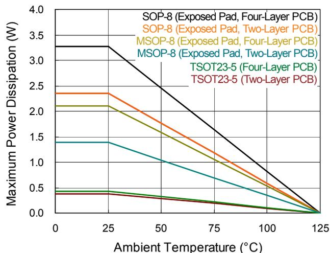
Figure 2. Derating Curves of Maximum Power Dissipation
