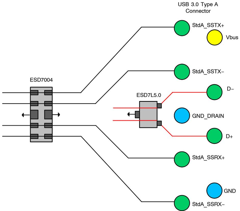
Figure 16. USB3.0 Standard A Connector Layout Diagram
