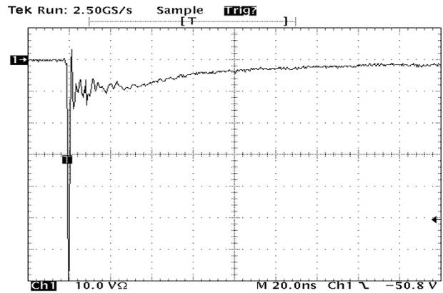
Figure 2. IEC61000-4-2 -8 KV Contact ESD Clamping Voltage
