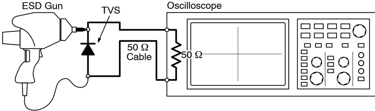
Figure 4. Diagram of ESD Clamping Voltage Test Setup
